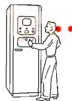
RCA Film Camera Monitor Rack. This is the control center of the projection room. It houses the amplifiers, all necessary rack-mounted power supplies, and the kinescope for viewing the film pictures.
