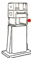
RCA Film Camera, Type TK-20A. A high-contrast film camera having unusual stability. It is used with either 16-mm or 35-mm film projectors, and slide projectors.
